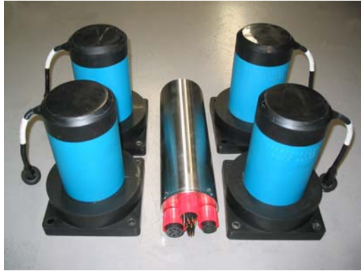
GeoChirp II subsea unit and 4 T135 transmit transducers
